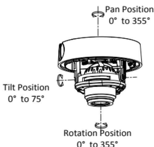
Figure 2-4 3-Axis Adjustment
