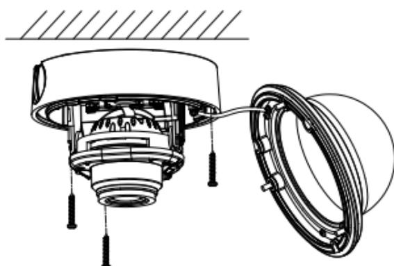
Figure 2-3 Attach the Back Box
