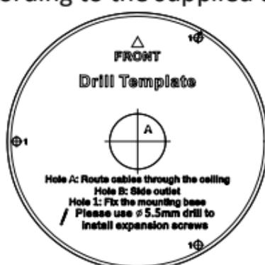
Figure 2-1 The Drill Template
