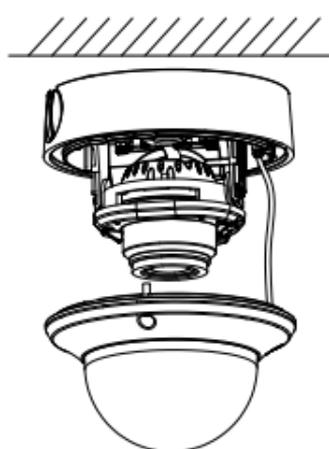
Figure 2-5 Fit the Black Liner Back
