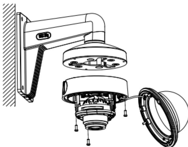
Figure 2-8 Attach the Back Box to the Mount
