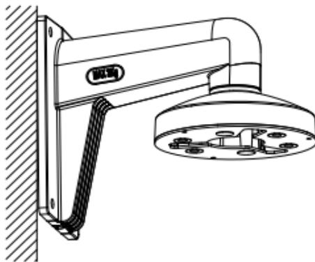
Figure 2-7 Install Wall Mount
