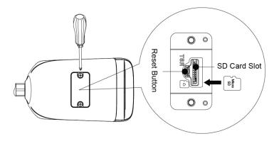
Press the reset button for 10 seconds to reset the device.
