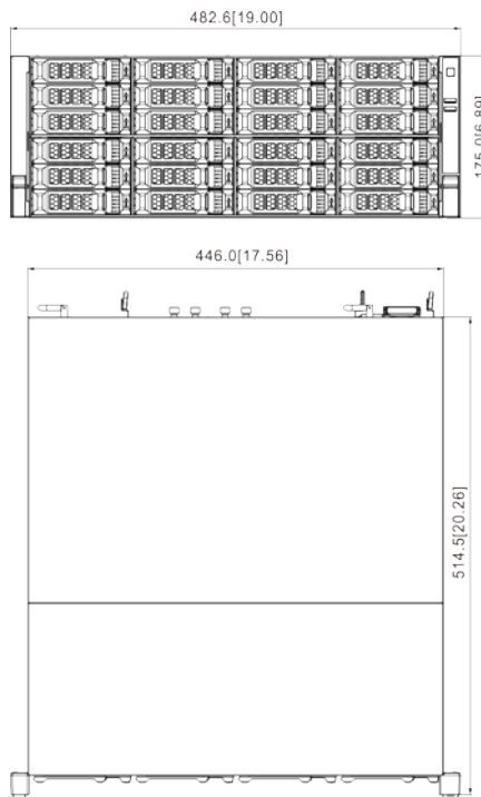
Figure 2-32 Dimensions without LCD (mm [inch])
