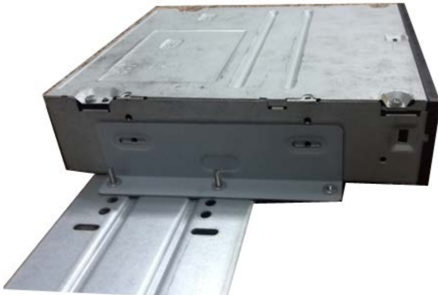
Figure 3-38 Install SATA burner
