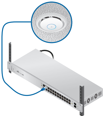
UniFi Switch Power Connection Diagram
