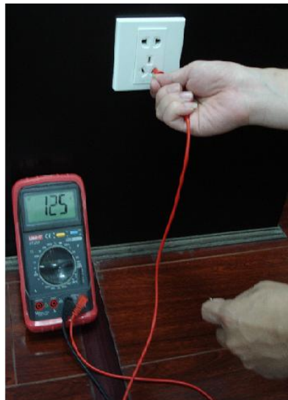
Appendix Figure 7-6 Check live cable connection
