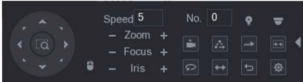
Figure 5-62 Expanded PTZ control panel
