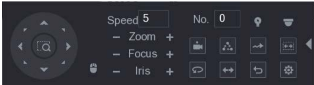
Figure 5-63 Expanded PTZ control panel
