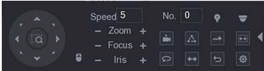
Figure 5-69 Expanded PTZ control panel
