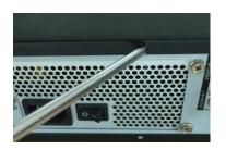
Loosen the screws of the upper cover and side panel. Remove the cover.
