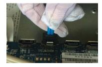
(4) Connect the other end of the HDD cable to the mainboard.
