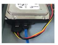
**(5)**Connect the HDD cable and power cable.
